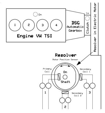
The resolver is mounted in the electric motor and consists of 3 coils
