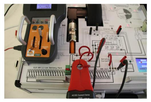
In this measurement, one phase was measured with the corresponding current. Probe settings: voltage probe x10, current probe x1000 (100mV / A).
