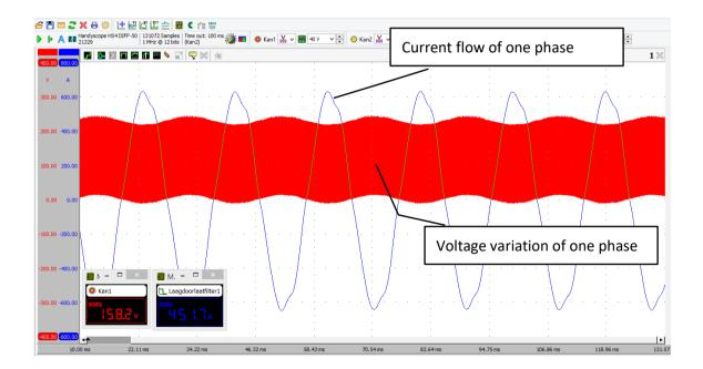
The voltage is switched by the Inverter via a high frequency (16 kHz). To get a good understanding of the voltage pulses, zooming is required.
