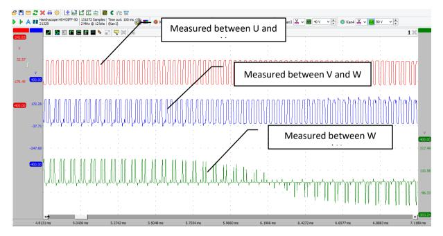
After magnification on the signals, a variable duty cycle is clearly visible.
