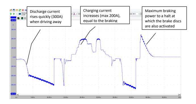
The property of an electric motor is that the maximum torque is present very quickly. There is some construction to prevent slipping. The correct probe setting shows the currents that are reasonably true to nature. Discharge currents run up to 300A and the regeneration current can be a maximum of 210A. In reality, the currents are 3A and 2.1A, respectively.
