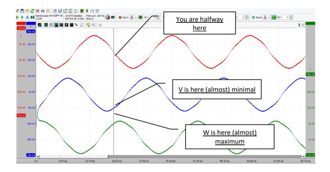
The measuring probes have an amplification factor of 10. The actual measured voltage will not exceed 24 Volts, but with this probe factor 10 setting the scale indicates 240 Volts. That is reasonably close to the actual voltage of 250 - 400 Volts of the applied battery.
