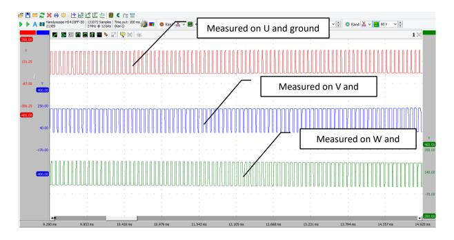
You can clearly see that the pulse width is constantly changing. With a broad pulse there is a relatively long voltage on the coil concerned and the current will also be high and the associated magnetic field will also be.
